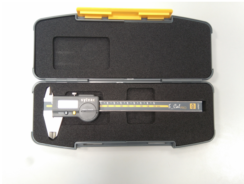
Figure 6 | Picture of the caliper used to measure the pieces. Photograph by the author.
