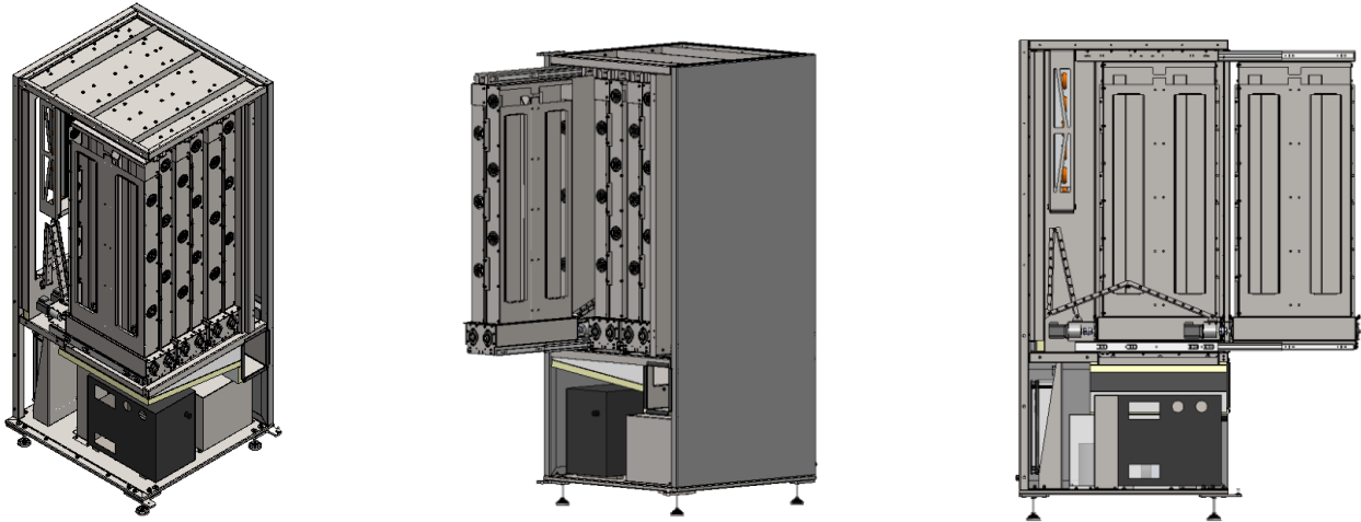
Figure 23 drawer system and cable management
