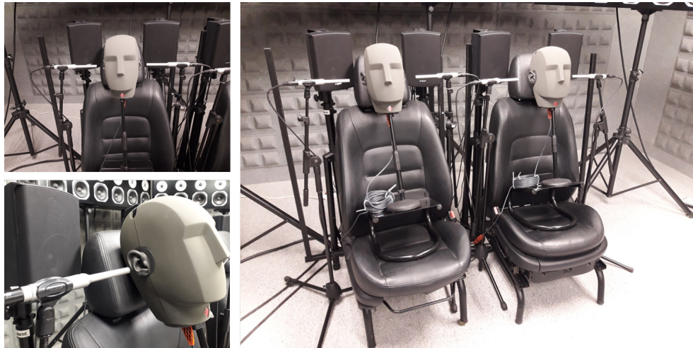
Figure 7.3: Three different views of the distributed SFC prototype mounted in the listening room of the Audio Processing Laboratory of the Polytechnic University of Valencia.
