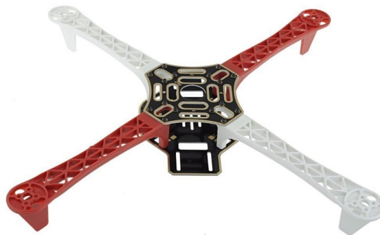
Figura 4.8: Chasis DJI F450
