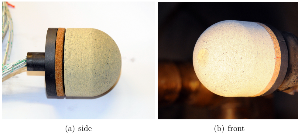
Figure 4.23: Virgin ZURAM ® sample used for the experiment prepared to be mounted and mounted in the VKI Plasmatron. Courtesy of Bernd Helber.
