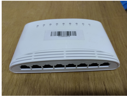
Figure 3.5: Switch to connect both cameras at the same computer to synchronize them.
