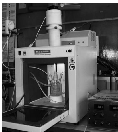
Figure 4. Simultaneous irradiation in a multimode MW oven equipped with a Pyrex horn [8].
