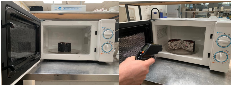
Fig. 1. Asphalt mixtures heating.
