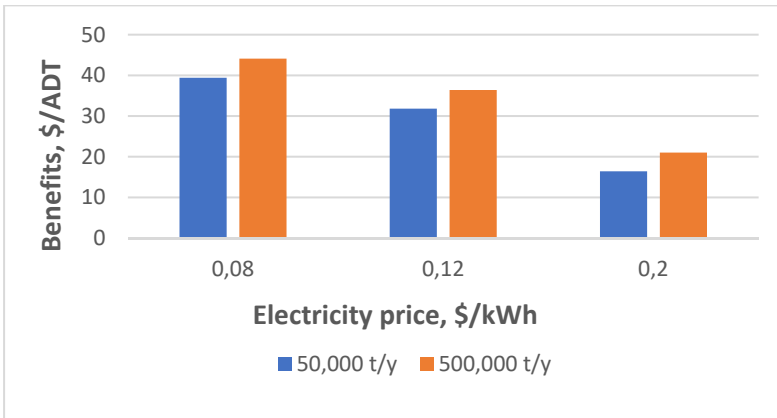
Fig.6. New MW technology benefits depending on electricity costs and pulp mill output.
