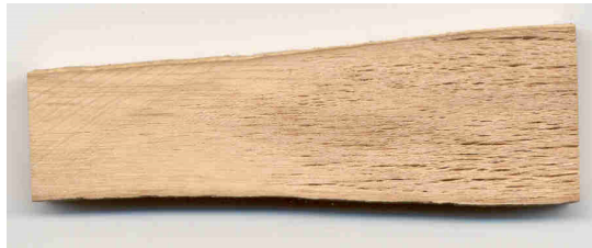
Fig 1. Wood sample after intensive MW modification. Left side - natural wood, right side - MW modified wood.
