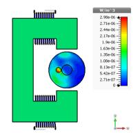
Fig. 5. power loss density in tissue in left-position.
