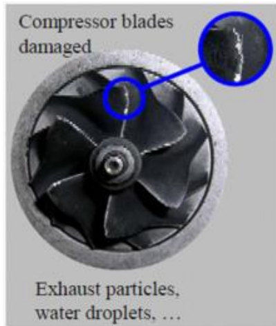
Figure 1.9: Compressor wheel damaged at CMT facilities after intensive LPEGR testing.
