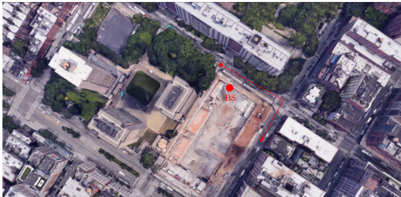
Figure 5.3: Satellite image from Google Maps of the zone considered in UMa. The location of the BS and the user walk path are visually represented by a red dot and a red arrow, respectively.
