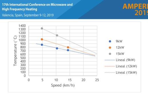
Fig. 14. Microwave power/peak temperature vs. Speed dependence, dielectric tube 3 mm
