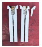
Fig. 5. Thermal shock damage of the AlN tube
