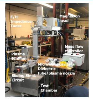
Fig. 3. Laboratory set-up
