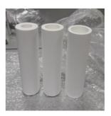
Fig. 6. BN machined tubes
