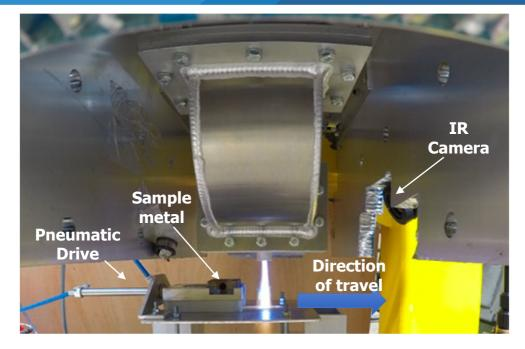
Fig. 9. Sliding shuttle & metal block
