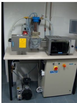
Fig. 1. Photo of a laboratory microwave vacuum station for testing drying processes. The device has been ordered by Institute of Fruit Farming in Skierniewice, Poland. Similar units have been delivered to several universities and research institutions and to industrial laboratories as well. Are mainly used for drying, but also for pasteurization and recently for seed structure modification. Very promising research has been carried out for drying of hemp before extraction.
