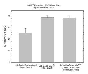
Fig. 3. Comparison of conventional extraction, lab-scale MAP<sup>TM</sup> Extraction and industrialscale MAP<sup>TM</sup> extraction of flax lignans (SDG) from flax biomass
