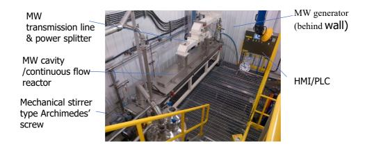
Fig. 2. Continuous-Flow Industrial-Scale MAP<sup>TM</sup> Extractor in ATEX environment
