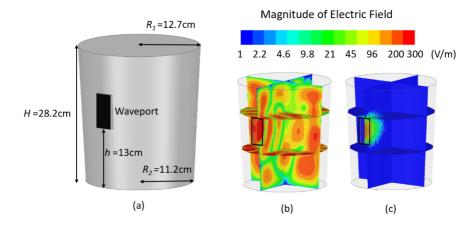
**Fig 2.** Simulated magnitude of the electric field for a single waveguide port excitation of a cavity completely filled with various materials. (a) Simulated cavity with dimensions labeled. (b) Cavity filed with food mixture  $\varepsilon_r = 42$  and  $\tan \delta = .3$ , and (c) Cavity filled with LDPE and polystyrene  $\varepsilon_r = 2.25$  and  $\tan \delta = .0003$ . The field value is normalized to a 1W incident power at 2.45 GHz on waveguide port.
