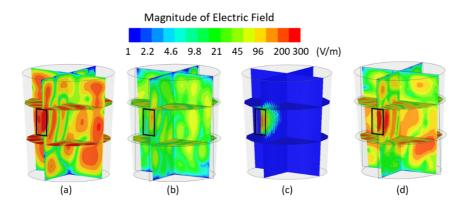
**Fig.1.** Simulated magnitude of the electric field, with 1W incident power at 2.45 GHz, inside cavities completely filled with (a) LDPE and Polystyrene,  $\varepsilon_r$  of 2.25, tan $\delta$  of .0003, thermal conductivity of .28 W/m°C, density of 950 kg/m<sup>3</sup> and specific heat of 2300 J/kg°C, (b)
