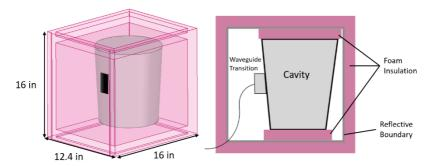
**Fig. 3.** Image of thermal simulation set up and a side cut of the insulation used in the simulation. The cavity filling is coupled to the field simulation as a thermal source. The cavity walls are 1mm thick tin-plated steel, the reflective surround has a reflectivity of 94% and the foam insulation is 1in thick XPS rigid polystyrene.
