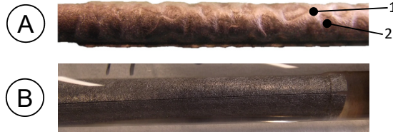
FIGURE 4.6: Heat bonded tubular MEAs with partially bonded GDE (A) and fully bonded GDE (B). 1: detached membrane section. 2: bonded section.
