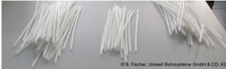
FIGURE 3.9: Picture of extruded VM-fumasep ® FFT membranes.
