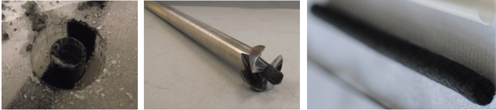
FIGURE 3.7: Left: frozen graphite sheet material. Middle: developed drilling tool with cylindrical electrode in the center. Right: cylindrical graphite felt electrode after fabrication.
