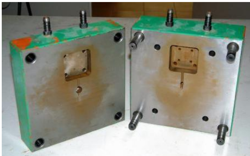
Figura IV-42. Portamoldes de dimensiones 100x100 mm.
