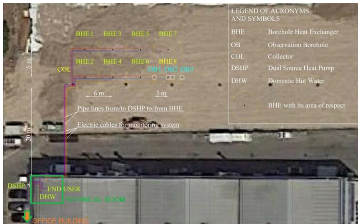
Figure 7. Map of the BHE field in the Tribano demo-site. Temperature sensors are located in OB 1, OB 2 and OB 3 (blue), as well as on the head of BHE8 and COL (yellow) [51]
