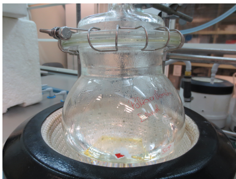
Figure 2.7: Glass flask containing the polymers immersed in a mixture of water and ethanol.
