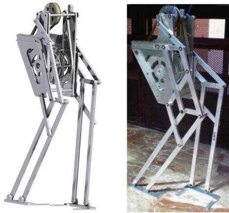
Fig. (1): the biped robot PASIBOT. Left: a virtual model. Right: the real prototype.
