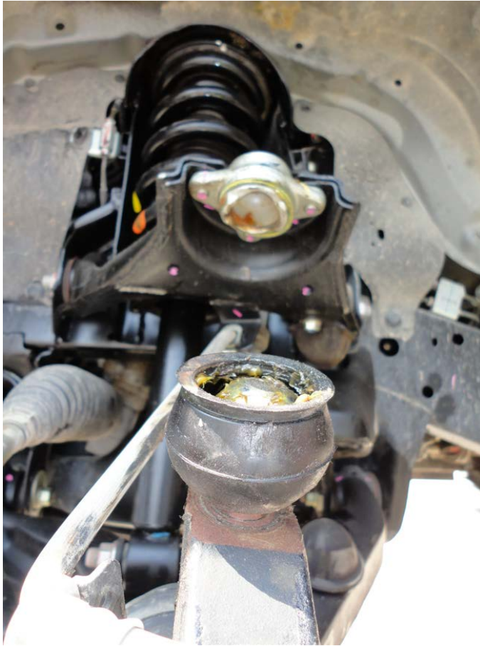
Photo No. 3 - in this photo you can see the ball joint covered by its poncho out of the cup.
