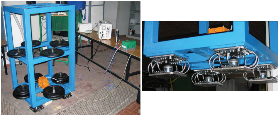
Figure 12 – Laboratory cabinet on WRS-BTU isolators
