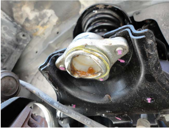
Photo No. 2 – Cup of the upper ball joint cup on the driver's side.
