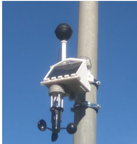
Figure 3. HSM - Heat stress monitoring box.
