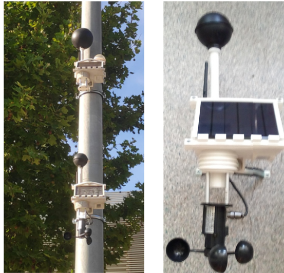
Figure 2. Proposed WBGT monitor prototype implementation
