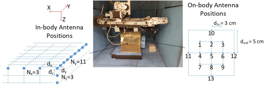
Figure 3.9: Measurement setup and in-body to on-body measured grid points
