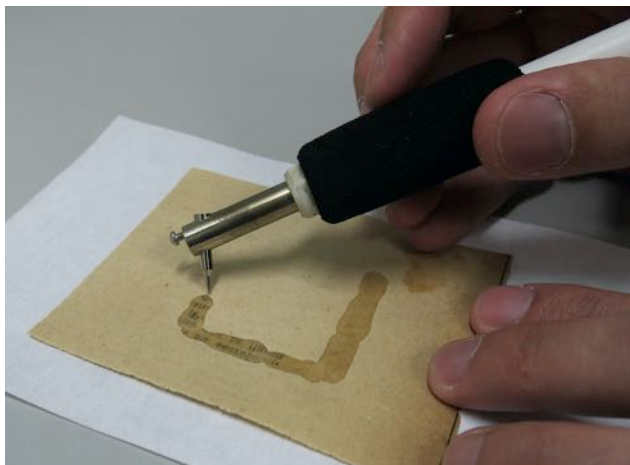
Figure 4: Melted CDD can spread through the paper in a way that is hard to control, thus producing thick lines that are inadequate for waterproofing thin lines or intricate shapes.
