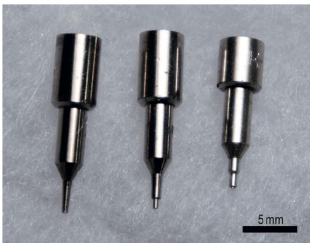
Figure 3: The tips used in the experiments. Following the manufacturer's nomenclature, the tips are, from left to right, tip #2, tip #1, and tip #00. The diameters of the tip holes are, respectively, 0.45 mm, 0.33 mm and 0.19 mm.
