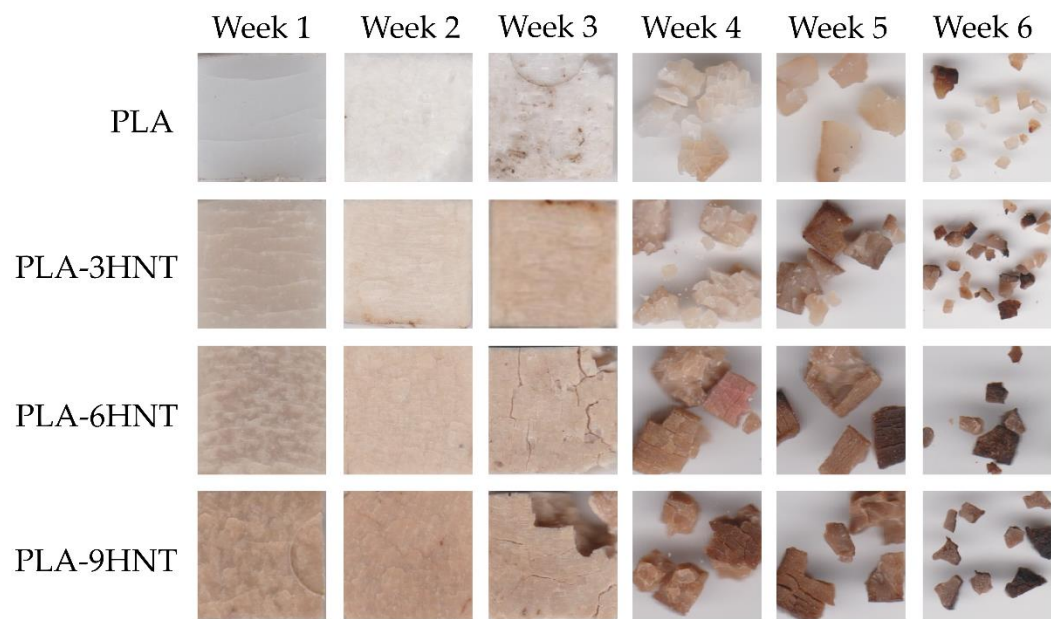
Figure III.2.10. Optical images of the disintegration in controlled compost soil of PLA-HNT composites with different HNTs loading.
