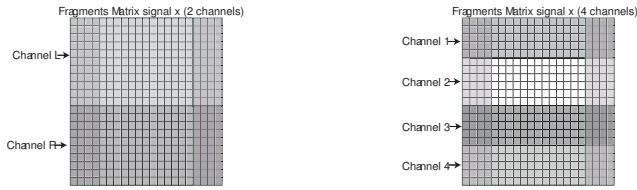
Fig. 7 Signal matrix on the left shows 2-channel resource sharing, signal matrix on the right shows 4-channel resource sharing
