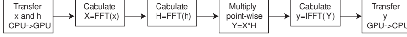
Fig. 2 Steps in order to calculate convolution of signals x and h on GPU.
