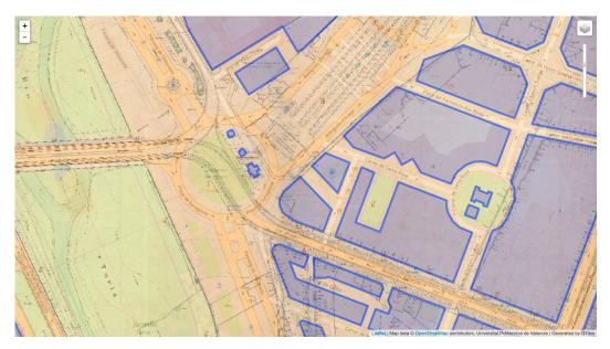
**Figure 7.** Screenshot of the viewer combining the 1929 map together with OpenStreetMap and vector data. The viewer allows replacing OpenStreetMap layer with an orthoimage.
