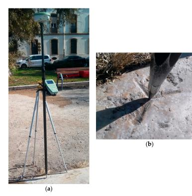
**Figure 4. (a)** The global navigation satellite system (GNSS) antenna and receptor during the resurvey of the vertex 86A; (b) the original mark of the vertex 86A.
