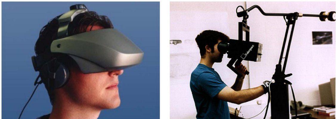
Fig. 2: HMD by 5DT (on the left) and BOOM by Fakespace (on the right).
