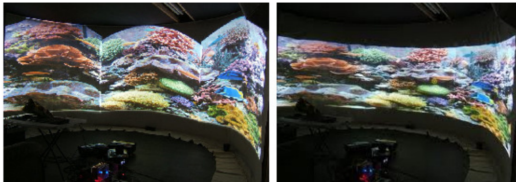
Fig 17: Three projectors without warping or blending on the left (a) and projections corrected (warped and blended) on the right (b). Done with Sol7 (Immersview) .
