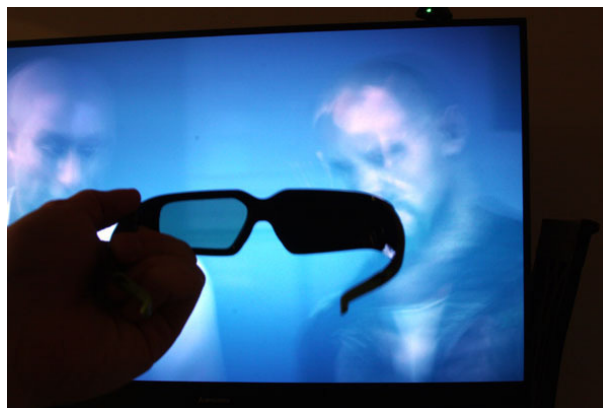
Fig 10: Shutter glasses working. Only one of the LCD glasses lets light through for a given instant.
