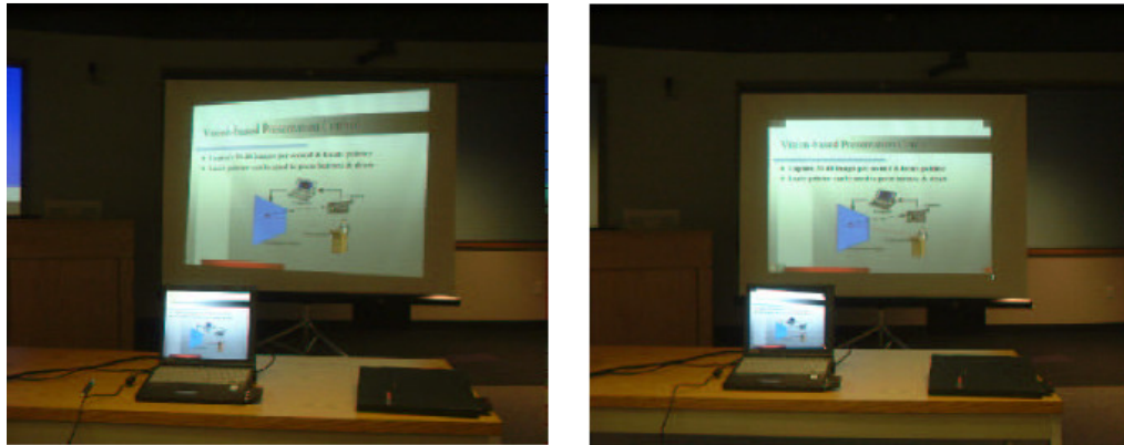
Fig 20: Image projected onto a screen without the correction applied (left) and applied (right). (Sukthankar, 2001 [13]).
