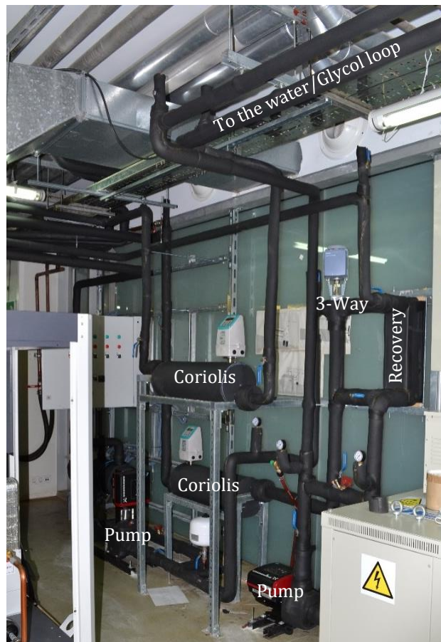
Figure A.5: Picture of the heat sink and source water loops on the test rig
