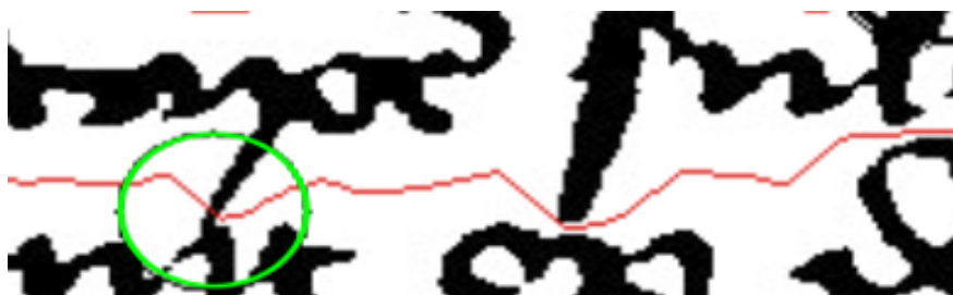
Figure 4.4: Section of sample frontier path that is forcefully required to cross through foreground pixels and the re-estimated circular frontier correction
