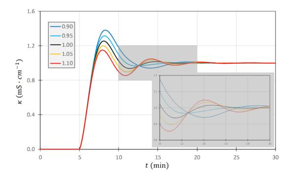
Figure 5: Effect of the error (e) in the gain of a non-ideal Smith's predictor  $(K' = e \cdot K)$  on the time evolution of the controlled variable (in deviation units)
