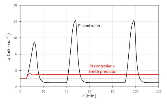
Figure 4: Comparison of the time evolution of the controlled variable (in deviation units) of a traditional PI controller versus a PI controller coupled with a Smith's predictor
