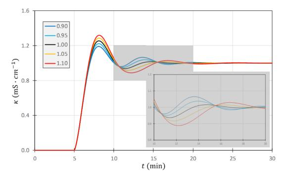
Figure 6: Effect of the error (e) in the time constant of a non-ideal Smith's predictor ( $\tau' = e \cdot \tau$ ) on the time evolution of the controlled variable (in deviation units)
