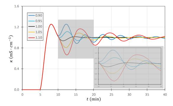
Figure 7: Effect of the error (e) in the time delay of a non-ideal Smith's predictor  $(b' = e \cdot b)$  on the time evolution of the controlled variable (in deviation units)
