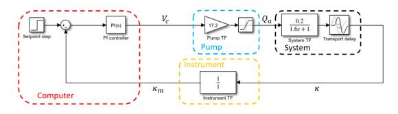
Figure 2: Simulink<sup>®</sup> model of the conductivity control system based on a PID controller
