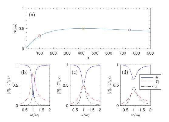
Figura 6: Analysis of the scattering parameters on the losses of the system. (a) represents the absorption of the system at the resonance frequency of the system as the losses increases. Dots in (a) represents the analyzed cases in (b), (c) and (d). (b), (c) and (d) show the scattering coefficients for three particular values of the losses:  $\sigma = 100 \text{ s}^{-1}$ ,  $\sigma = 416 \text{ s}^{-1}$ ,  $\sigma = 750 \text{ s}^{-1}$  respectively.
