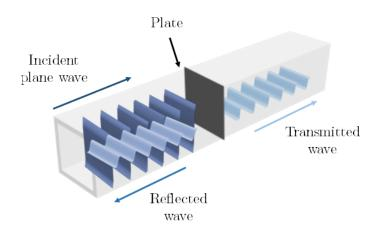
Figura 1: 3-D scheme of the problem in transmission. Dark blue represents the incident plane wave generated by the source, medium blue represents the sound wave that is reflected by the plate and soft blue represents the transmitted wave. The plate is represented in grey.
