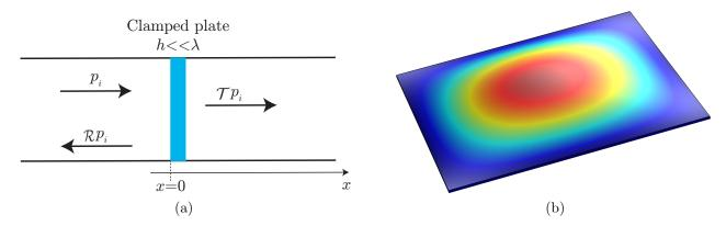
Figura 2: (a) 1-D scheme of the problem in transmission. (b) First mode (piston mode) of the plate.
