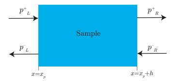
Figura 4: Forward and backward waves in the scattering process.
