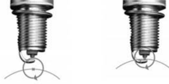
Figure 2.2. Origin of the combustion cyclic variability. Source: [1].
