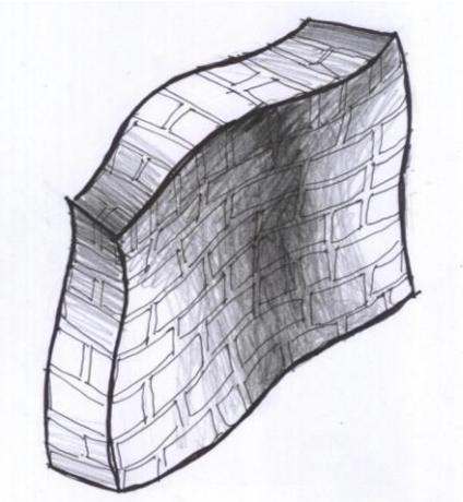
*Fig. 5 The deformation in a curvilinear form, since the material is tired and is bending with the load*
