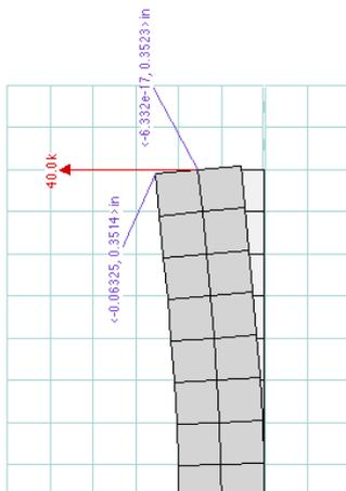
Fig. 12 Dead constant load of the brick, and bucking effect due to torque
