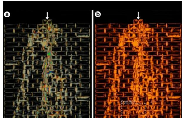
Fig. 21 The electrolysis analysis of the salt travel on the Moen-Jo-Daro wall.
