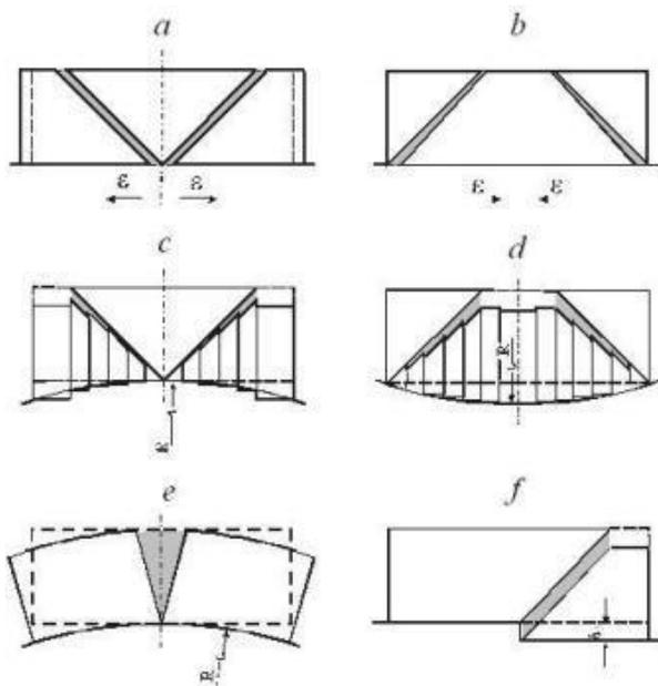
Fig. 7 The generalized structural deformations of the walls induced by: a – horizontal shear due to ground surface tension; b – horizontal shear due to the ground surface compression; c – vertical shear due to the curvature of convexity; d – vertical shear due to the curvature of concavity; e – bending due to the curvature of convexity; f – vertical shear due to the bench formation
