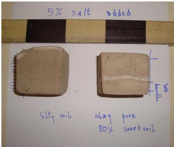
Fig. 22 Experiment of submerge the clay cube into salted water.
