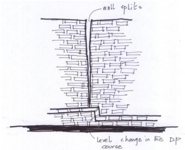
Fig.26 The elevation diagram of the wall
