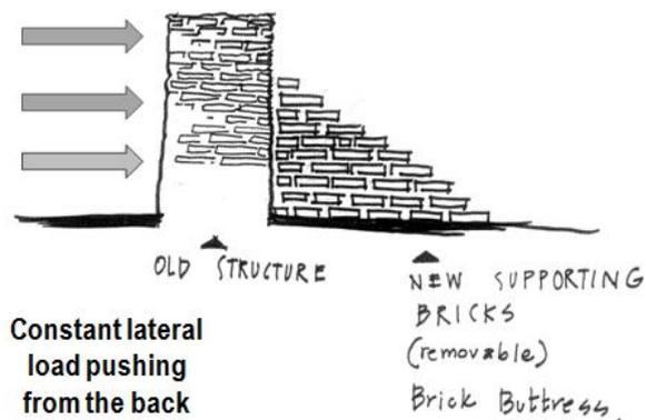
*Fig. 2 The brick are being attacked by the salted water from the back, of the inclining wall*
