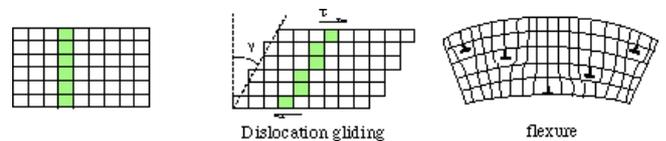
Fig. 9 The deformation patterns of buildings and indexes of deformation due to the tension and the curvature of convexity
