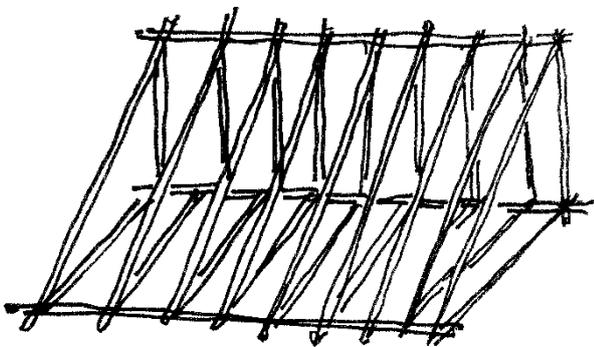
*Fig. 14 individual Bamboo truss, mobile design, simple low cost solution, to support the falling wall.*
