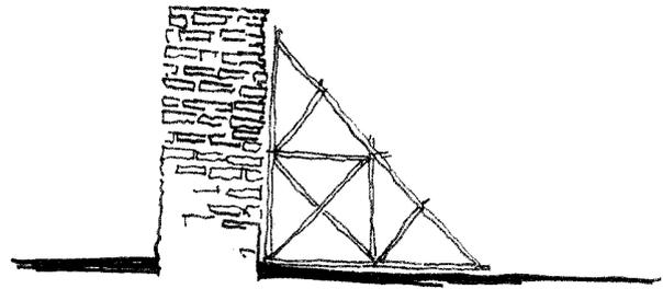
*Fig. 15 the instillation of the buttress to support the falling wall*
