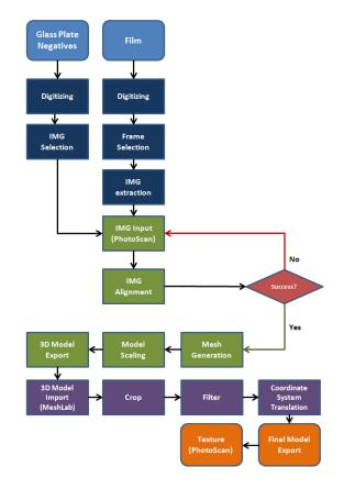
Fig. 1 Process Work Flow
