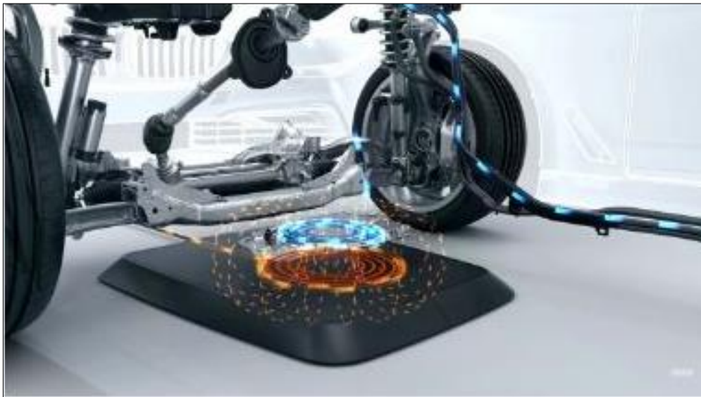
Fig. 3 Induction charging system
