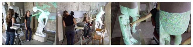
Figure 2: The acquisition process. The string helps to keep the camera at the same distance from the chosen surface point. The camera autofocus is switched off both for greater speed and accuracy.
