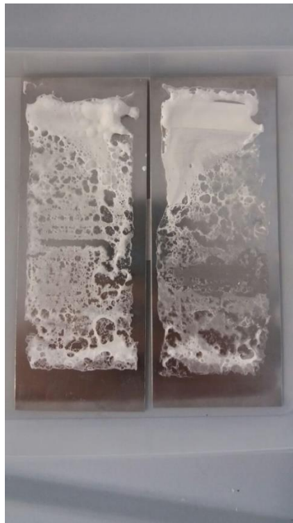
Figure 4.32 Tapes compound of alginate and COK-12 with different compositions: A) T_Alg90_OMS10(400)_8%, B) T_Alg95_OMS5(400)_8%.
