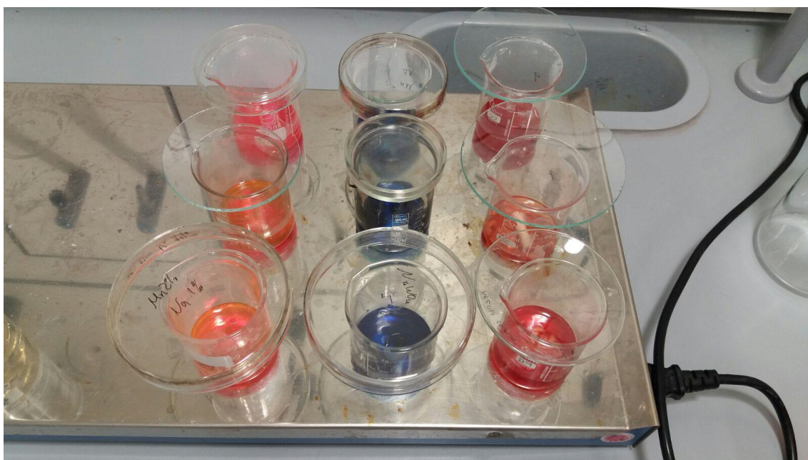
Figure 3.7 Solutions of methylene blue, rhodamine 6G and congo red stirred with different adsorbants: COK-12_500, S_Alg_OMS(500)_8%_N2, S_Alg_OMS(500)_8%_CaCl2.
