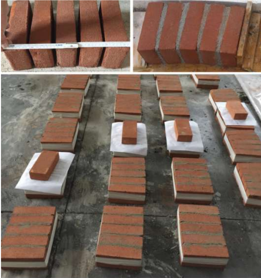
Figure 8: Manufacturing of masonry specimens
