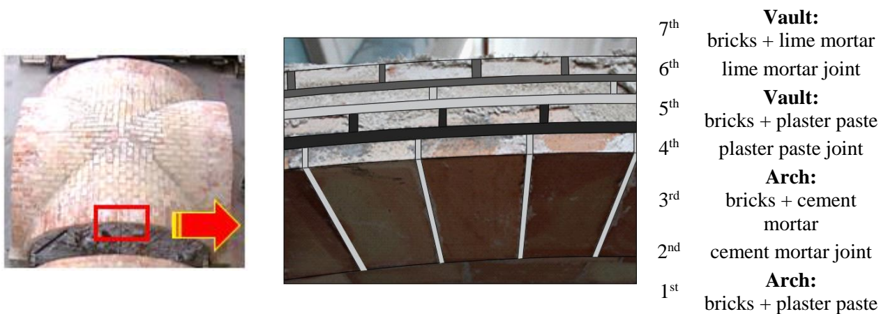
Figure 8: Masonry cross vault: detail of one of the arch.
