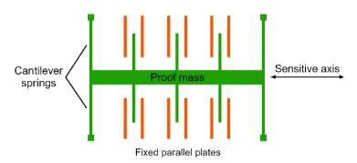
Figure 2: MEMS principle of operation
