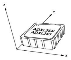
Figure 5: Axes of Acceleration [4]
