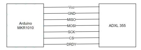
Figure 12: Scheme of connection between microcontroller and accelerometer
