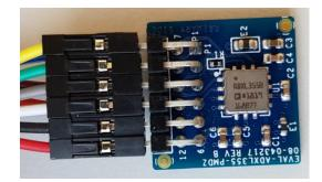
Figure 3: Accelerometer ADXL355
