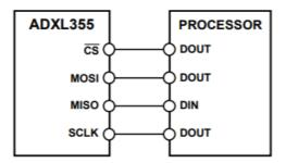
Figure 7: 4-wire SPI connection [4]
