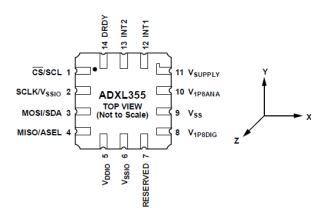
Figure 4: Accelerometer - Pin Configuration [4]
