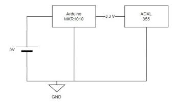
Figure 14: power supply scheme
