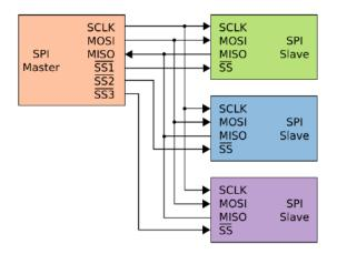
Figure 6: SPI master slave communication protocol
