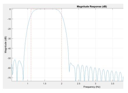
Figure 25: Algorithm 1- bandpass filter
