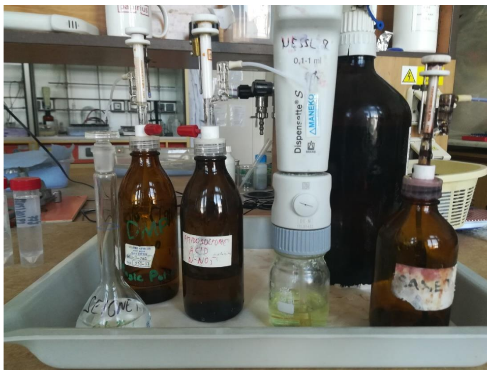
Figure 9. Reagents which are used to carry out the nitrogen/kinetic test of the collected samples: accumulation, reactor and effluent. Source: author.
