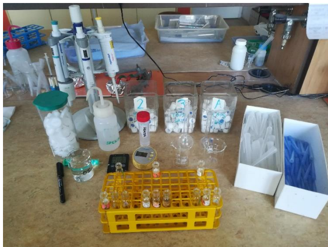
Figure 13. Necessary instruments for carrying out the kinetic test of the reactor sample from the pilot plant every hour. Source: author.
