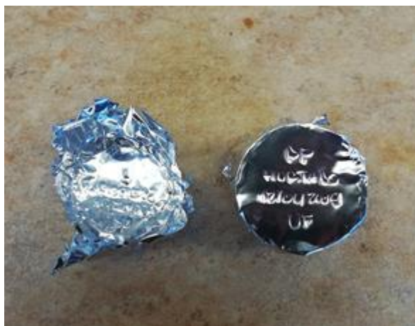
Figure 17. Piece of aluminium foil referenced where the reactor sample is poured: 1x filtered sample and 1x homogenized sample. Source: author.
