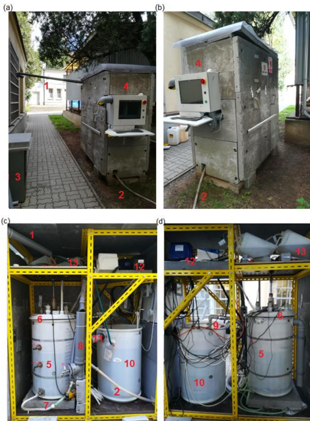
Figure 7. Pilot plant located in University of Chemistry and Technology, Prague (UCT) and used in the research of partial nitrification reaction which takes part in PN/A process for nitrogen removal in sewage: a) front part, b) back part, c) inside of front part, d) inside of back part. Source: author.
