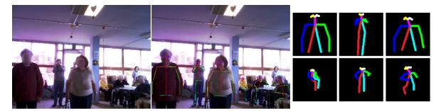
**Figure 2.** Human representation in terms of limbs by using Openpose: (**left**) Original image taken by the Pepper robot; (**middle**) Openpose output as body keypoint coordinates; (**right**) The human skeleton colour-coded to properly distinguish each limb (one per person).
