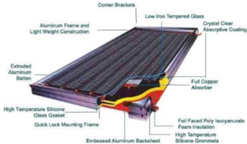
Figure 2.2: Components of flat plate solar collector
