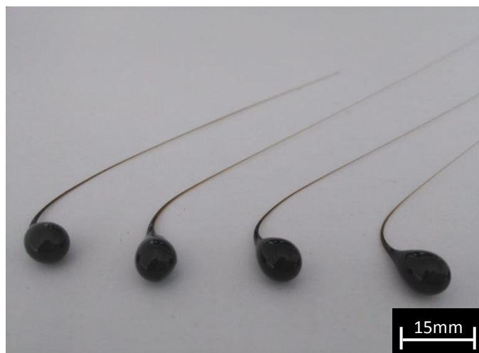
Figure 6.6: Some of the recovered droplets from ITALUS-1 with fiber formation
