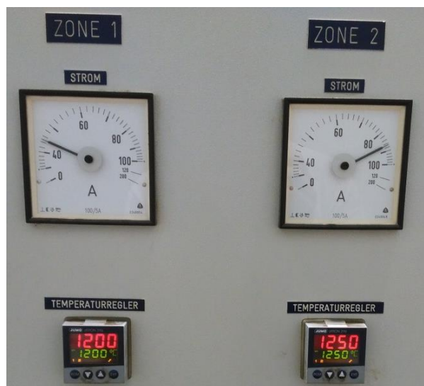
Figure 6.2: Working temperature in the lower part (left) and at the upper part (right) of the oven. ITALUS-1
