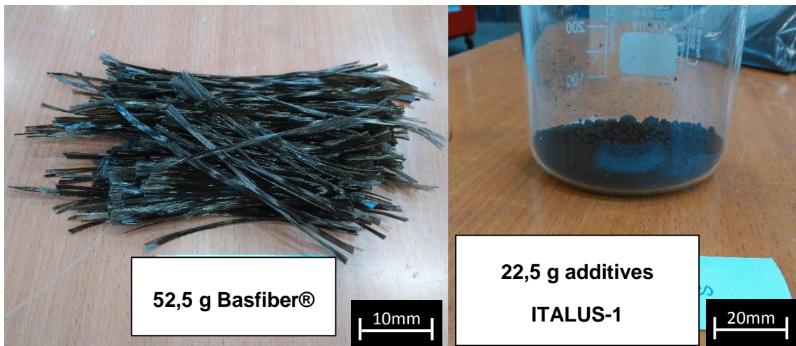
Figure 5.6: Base material and additives for a 75 g ITALUS-2 sample
