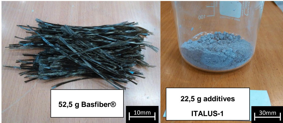
Figure 5.4: Base material and additives for a 75 g ITALUS-1 sample. Additives
