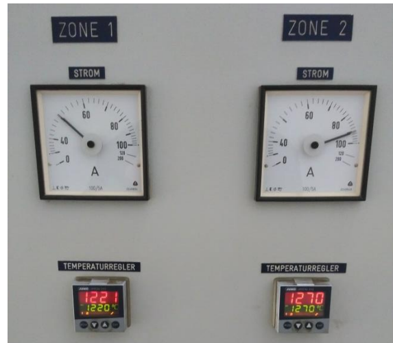
Figure 6.4: Working temperature in the lower (left) and at the upper (right) spinning machine's heaters. ITALUS-2
