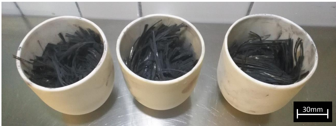
Figure 5.7: Three batches of ITALUS-2 before melting
