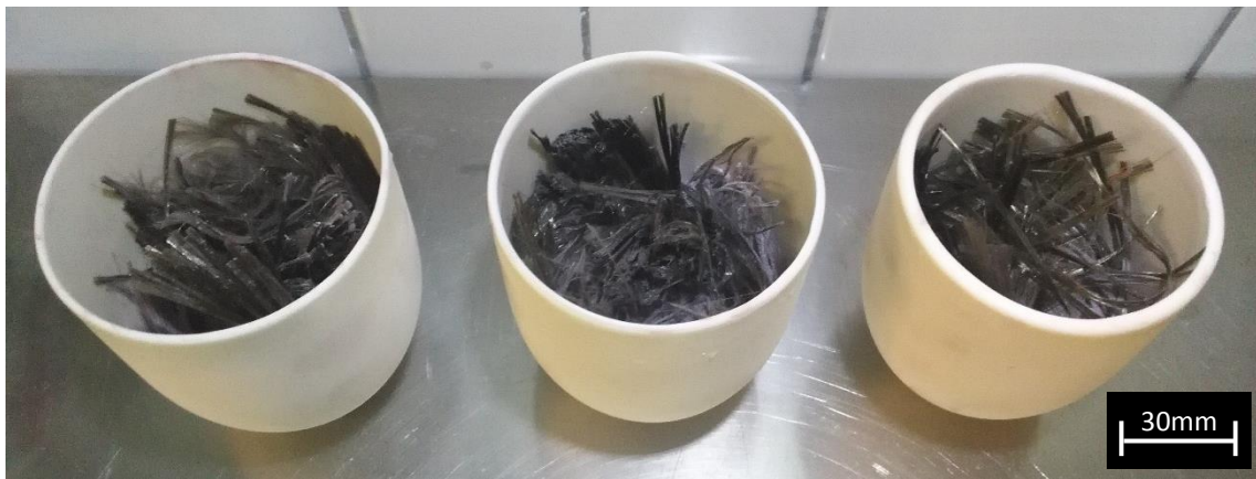
Figure 5.5: Three batches of ITALUS-1 before melting
