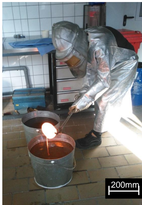
Figure 5.10: Pouring the melted ITALUS-1 into water
