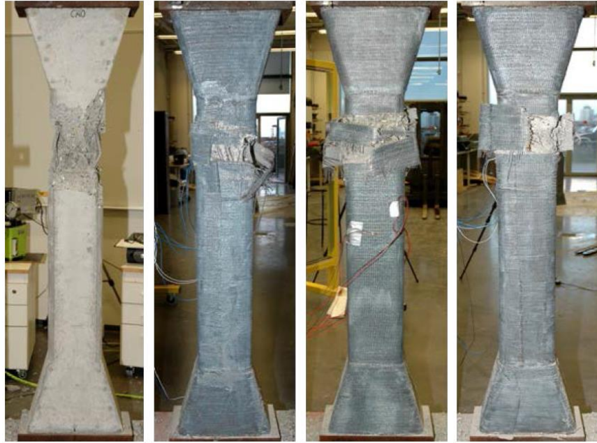
Figure 7.1. Renovation of concrete columns by wrapping basalt fiber sheets. [Tho13]
