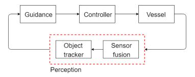
Figure 3.2: General structure for the USV system
