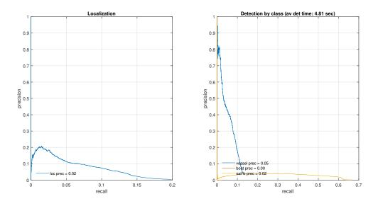
Figure 4.33: Precision-recall curve for ACF detector
