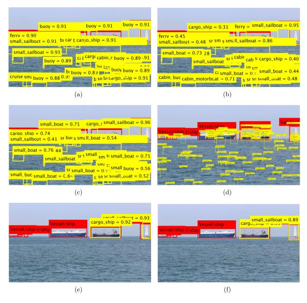
Figure 4.30: Object detection on SMD visible video sample frame: (a) ROI + SVM; (b) ROI + CNN (Alexnet); (c) ROI + CNN (VGG16); (d) ACF; (e) Faster RCNN (AlexNet); (e) Faster RCNN (VGG16)
