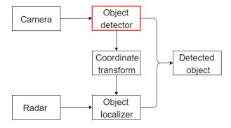
Figure 3.4: Scheme for the sensor fusion module
