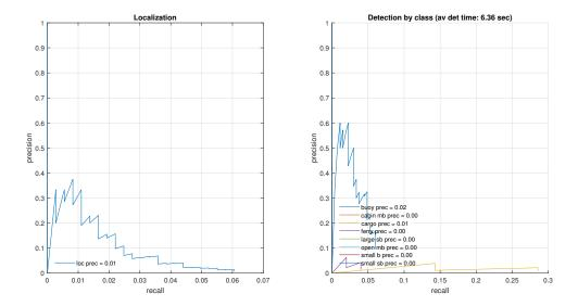
Figure 4.27: Precision-recall curve for ROI finder + CNN classifier (AlexNet)
