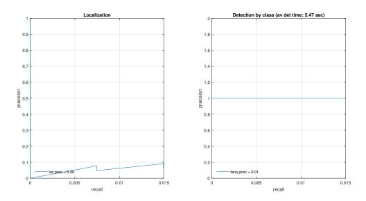
Figure 5.6: Precision-recall curve for ACF detector
