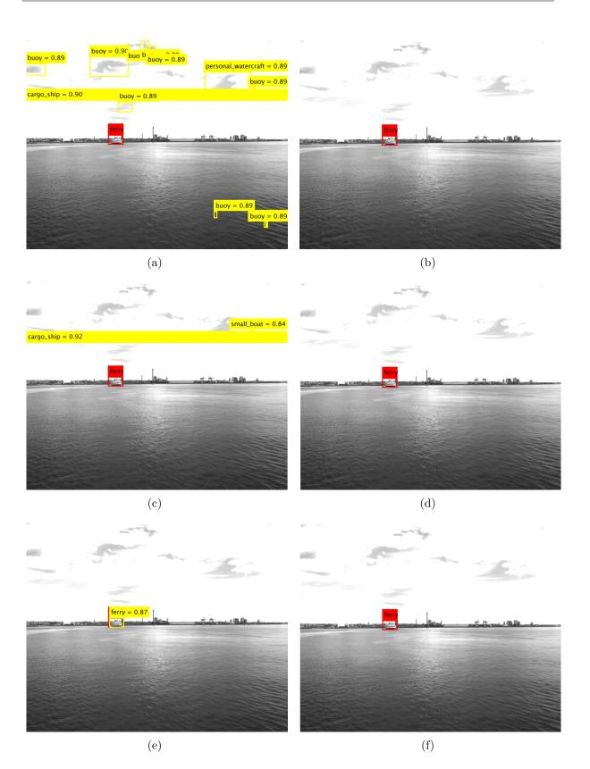
Figure 5.5: Object detection on Helsingor sample monochrome image: (a) ROI + SVM; (b) ROI + CNN (Alexnet); (c) ROI + CNN (VGG16); (d) ACF; (e) Faster RCNN (AlexNet); (e) Faster RCNN (VGG16)
