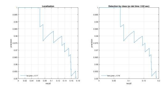
Figure 5.3: Precision-recall curve for Faster RCNN detector (AlexNet)
