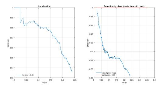
Figure 4.34: Precision-recall curve for Faster RCNN detector (VGG16)
