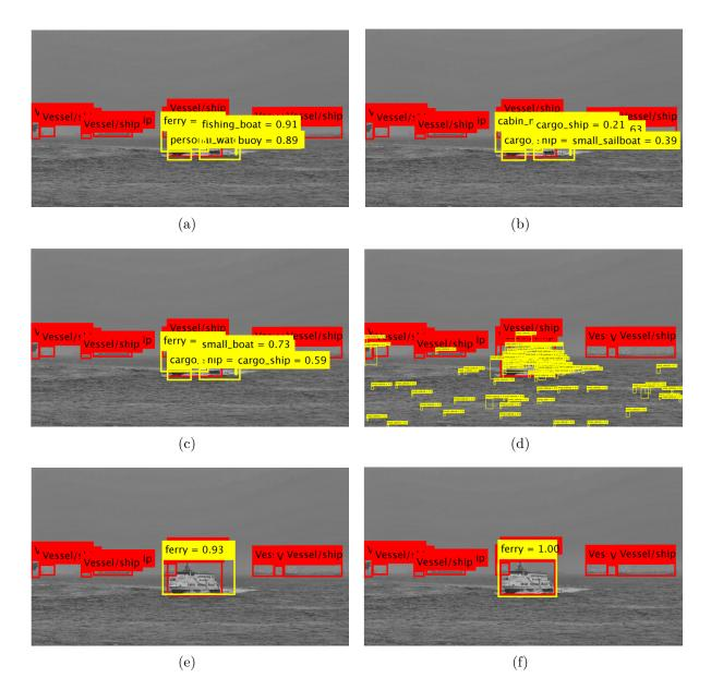
Figure 4.35: Object detection on SMD NIR video sample frame: (a) ROI + SVM; (b) ROI + CNN (Alexnet); (c) ROI + CNN (VGG16); (d) ACF; (e) Faster RCNN (AlexNet); (e) Faster RCNN (VGG16)
