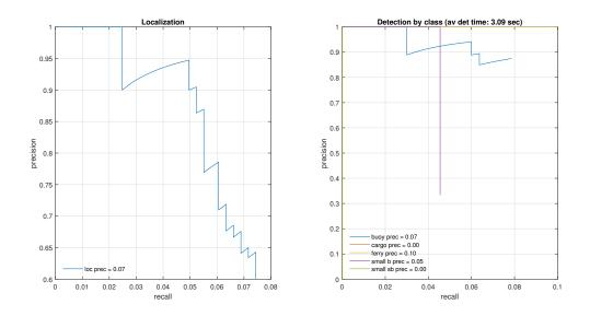
Figure 4.29: Precision-recall curve for Faster RCNN detector (AlexNet)
