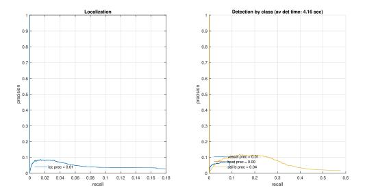
Figure 4.31: Precision-recall curve for ROI finder + CNN classifier (AlexNet)
