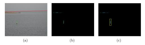
Figure 4.17: ROI algorithm for buoy localization: (a) Horizon line detection; (b) Background subtraction; (c) Region of Interest
