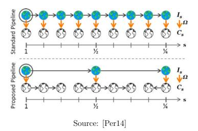
Figure 4.9: Fast feature pyramid working principle compared to standard feature pyramid computation
