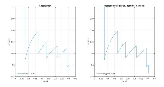
Figure 5.8: Precision-recall curve for Faster RCNN detector (VGG16)
