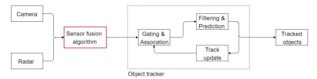
Figure 3.3: Scheme for the object detection and tracking system
