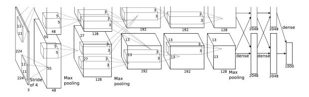
Source: medium.com/@smallfishbigsea/a-walk-through-of-alexnet-6cbd137a5637 Figure 4.13: AlexNet architecture
