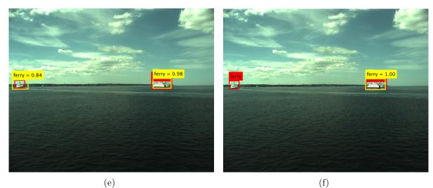
Figure 5.1: Object detection on Helsingor sample color image: (a) ROI + SVM; (b) ROI + CNN (Alexnet); (c) ROI + CNN (VGG16); (d) ACF; (e) Faster RCNN (AlexNet); (e) Faster RCNN (VGG16)
