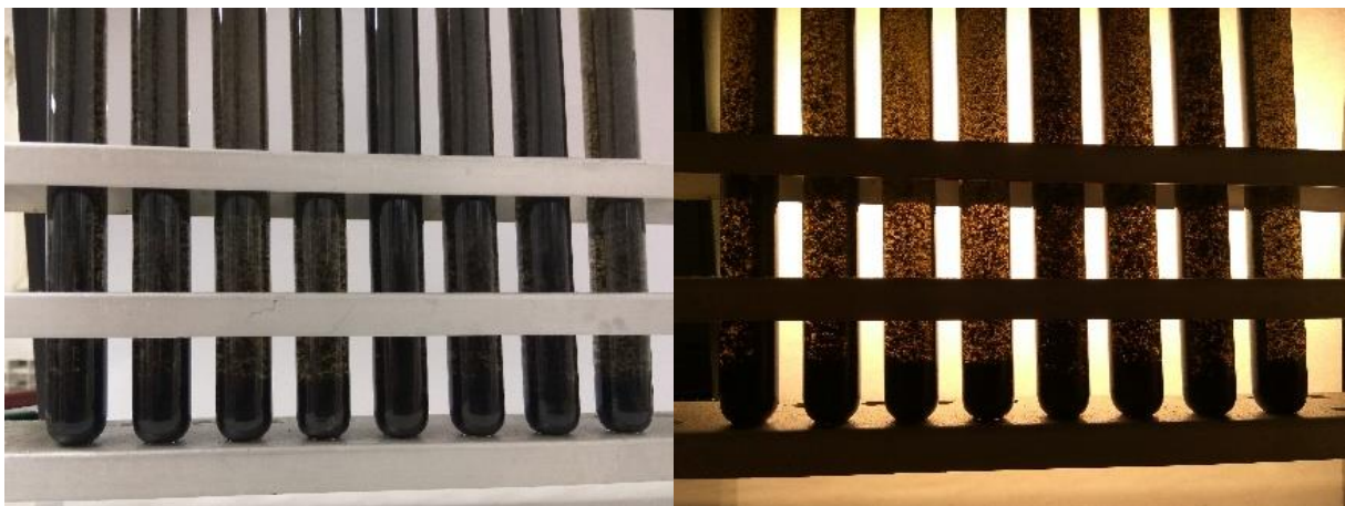
Figure 4-4 Nanofluids based on MWCNT Day 1, left to right (DF0 0.5%, DF2.5 0.5%, DF5 0.5%, DF10 0.5%, DF2.5 0.1%, DF5 0.1%, MD0 F5-K3 0.1%, SD0 F5- K1.9 0.1%)
