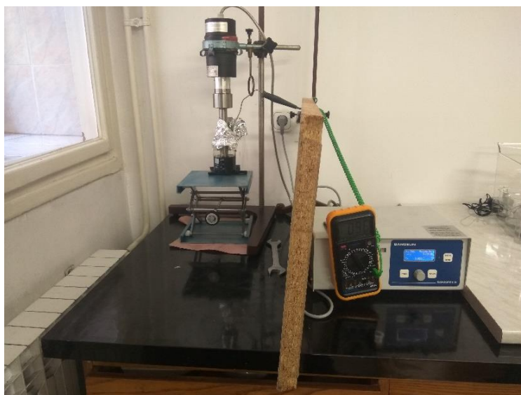
Figure 3-1 Ultrasonic device used to disperse nanomaterials
