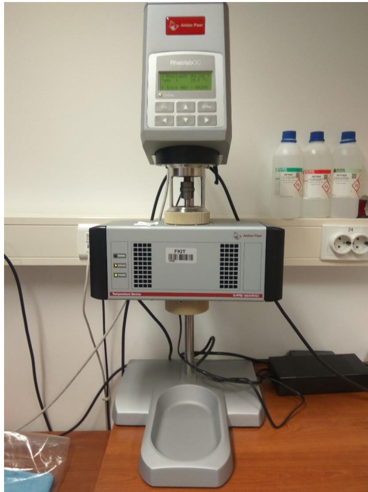
Figure 3-3 The Anton Paar Rotational Rheometer RheolabQC ©
