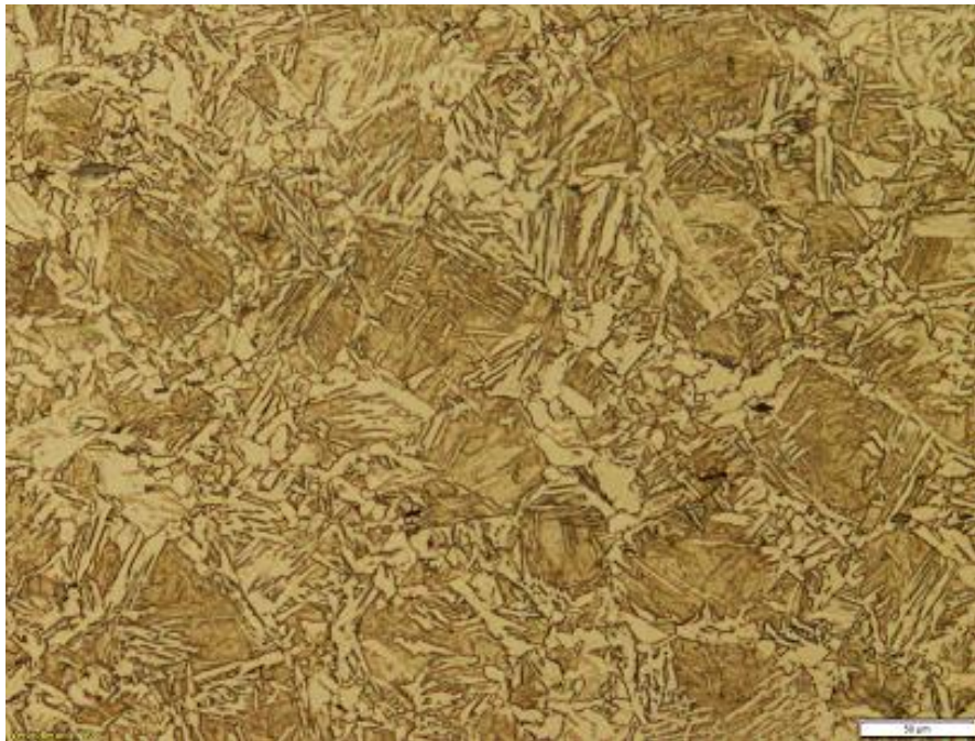
Figure 4.12 H.A.Z. magnification 20x (the white field equals 50 micrometres); Etched with "2% \text{HNO}_3 " etching agent.
