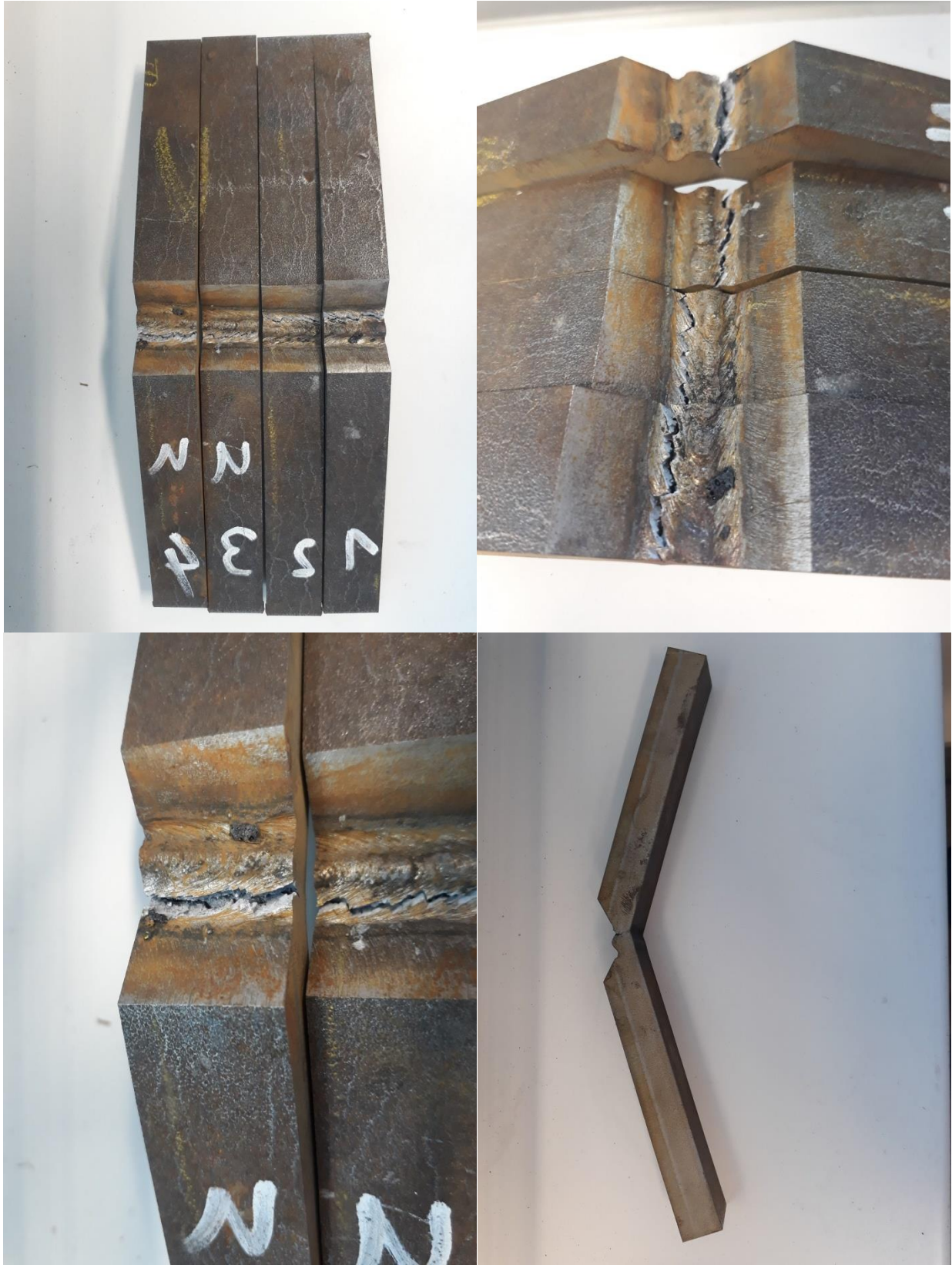
Figure 4.3 Bending test probes after the test.
