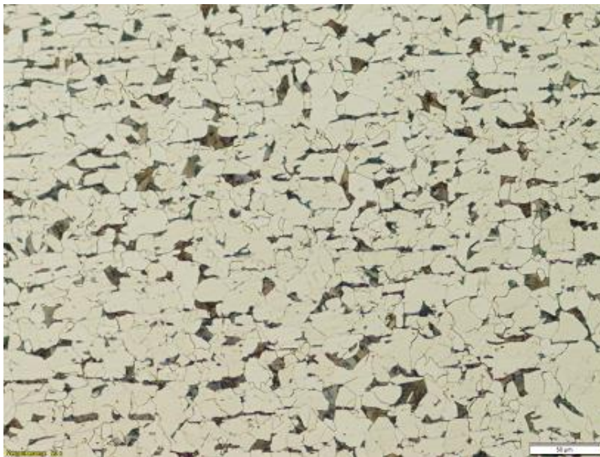
Figure 4.10 Base metal magnification 20x (the white field equals 50 micrometres); Etched with "Beraha 1" etching agent.
