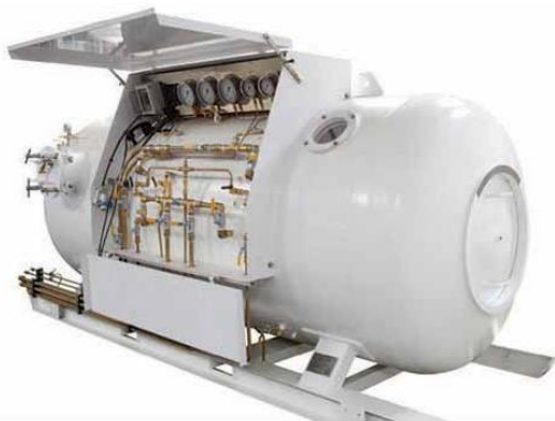
Figure 2.2: Hyperbaric Chamber used for dry underwater welding.
