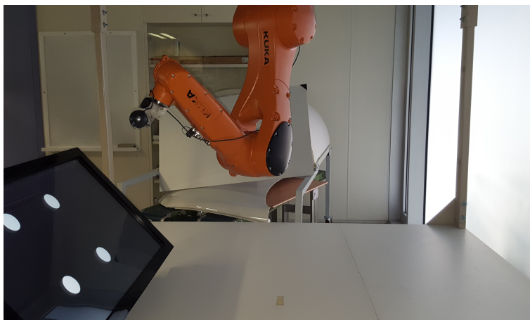
Figure 13. Experimental setup: 6R serial industrial manipulator in ceiling position with the camera rigidly attached to the robot end-effector (eye in hand configuration) and a screen to display the object markers.
