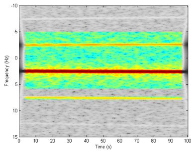
**Figure 7.** Example of t-f spectrum where the range of frequencies that would be necessary to obtain broken bar fault features has been marked.
