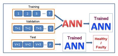
**Figure 10.** Scheme about training and classification for *X* iteration in the *'training/validation/test cross validation'* training algorithm.
