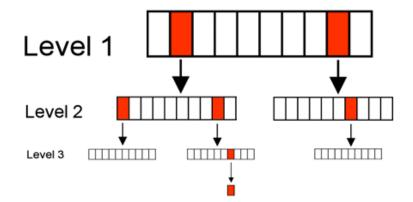
Figure 8. Schematic example of setting a parameter with the mesh search method.
