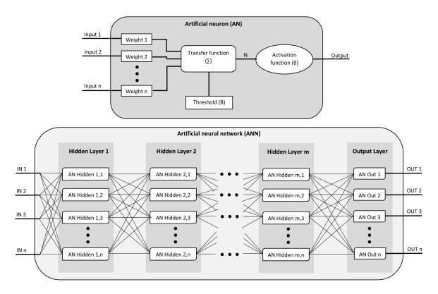
Figure 4. Scheme of Multilayer Perceptron neural network.
