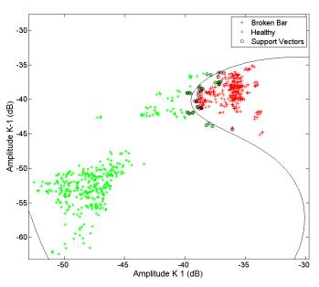
**Figure 3.** Space of a 2-dimensional SVM (2 parameters on each failure representative feature) where a hyperplane is splitting the space in subspaces of healthy features and failure features.
