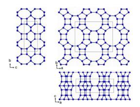
Figure 2. Structure of the zeolite ITQ-62. View along the main crystallographic axes. Oxygen atoms have been removed for clarity.
