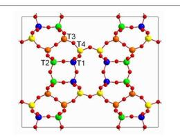
Figure 4. Location of the Ge atoms in the ITQ-62 structure. T1: 34 atomic % Ge, T2: 29 %, T3: 0 %, T4: 12 %.
