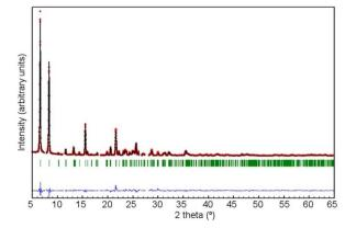
Figure 1. Rietveld refinement of the X-ray diffraction pattern of calcined ITQ-62. Red data points show the observed XRPD pattern; the black line along these points is the calculated XRPD pattern, with the difference profile at the bottom in blue. The green vertical ticks give the positions of the Bragg reflections. Residual values:  $R_{wp}$ =0.153,  $R_{exp}$ =0.047,  $R_{B}$ =0.069 and  $R_{r}$ =0.072. Wavelength corresponds to Cu K $\alpha$
